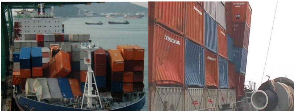
Container loss occurred by the green water loading
