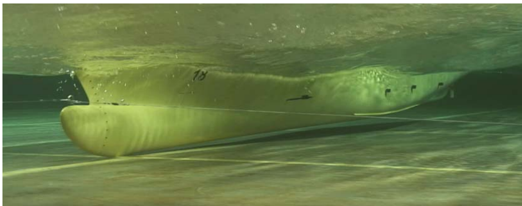
The model bulb hits the basin floor (time on video 11968 s) ( H_s = 6.5 m, T_p = 13.2 s, beam waves, zero speed)
