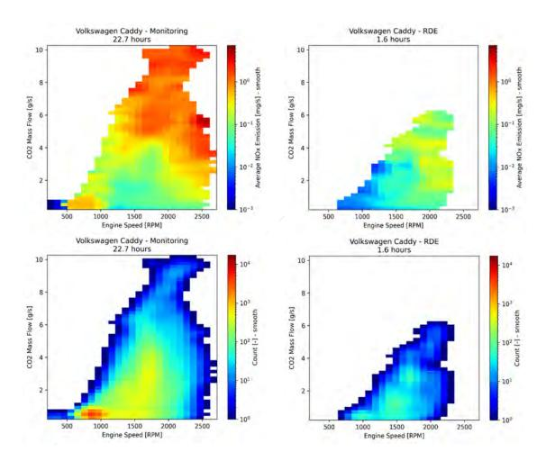
Figure C-1: The upper figures show coverage of engine operation during 22.7 hours of on-road emission monitoring and a RDE trip of the Euro 6d diesel Volkswagen Caddy. The bottom figures show the count of occurrences in certain engine operating points.
