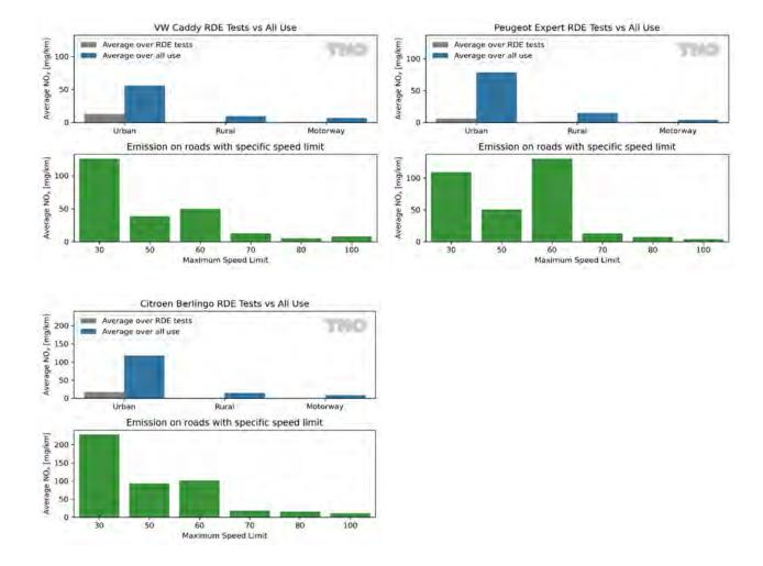
Figure 3.2: A comparison of RDE NO<sub>x</sub> emission results versus all-use (monitoring) emission results, subdivided per road type. There is a significant difference in the RDE results and all-use results. Also the all-use average NO<sub>x</sub> emission results per speed limit is shown. All three vehicles have consistently low NO<sub>x</sub> emission on roads with a speed limit of 70 to 100 km/h.
