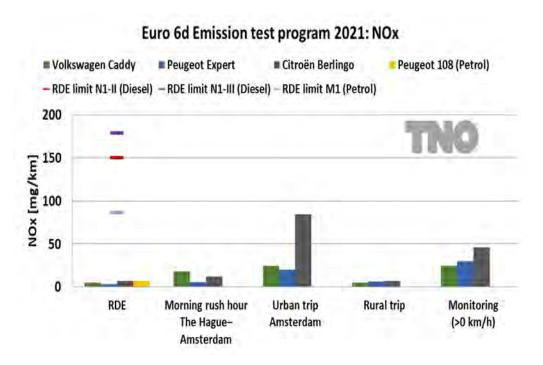
Figure 3.1: NO<sub>x</sub> emission results per test trip of the emission test program for three Euro 6d diesel vehicles and one Euro 6d petrol vehicle. The Peugeot 108 petrol was measured with PEMS and did not participate in the emission test program besides the RDE trip. The RDE trips for the diesel vehicles include a hot start and the RDE trip for the Peugeot 108 include a cold start.
