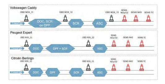
Figure 4.1: Schematic overview of the position of catalysts, in-vehicle NO<sub>x</sub> sensors and installed SEMS sensors (in red) in the exhaust pipes of the three tested Euro 6d diesel vehicles. For each vehicle the in-vehicle NO<sub>x</sub> sensors (named 'OBD NOX\_1x') have a different position in the exhaust pipe. Only the in-vehicle NOx sensor ('OBD NOX\_13') of the Volkswagen Caddy is measuring actual tailpipe-out NOx emissions.
