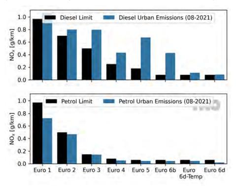
Figure 1.1: NO<sub>x</sub> Emission factors for urban traffic and type approval limit values of Euro 1-6 diesel (top) and petrol (bottom) M1 & N1 Class 1 vehicles.
