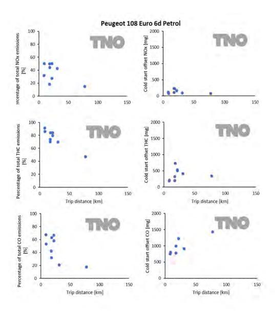
Figure 3.6: Cold start NO<sub>x</sub>, THC and CO emissions of an Euro 6d Peugeot 108 petrol as a percentage (left) of the total trip emission for varying trip distances and absolute cold start NO<sub>x</sub>, THC and CO emissions (right) in relation to their trip distance. Each dot represents a single cold start trip.
