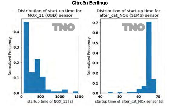
Figure 4.5: Monitoring data of the Euro 6d Citroën Berlingo. On the left: distribution of start-up times of the invehicle NOx sensor (pre-ASC). On the right: distribution of start-up times for the SEMS NOx sensor.
