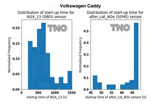
Figure 4.2: Monitoring data of the Euro 6d Volkswagen Caddy. On the left: distribution of start-up times of the in-vehicle NO<sub>x</sub> (tailpipe-out). On the right: distribution of start-up times for the SEMS NO<sub>x</sub> sensor.
