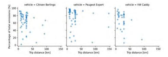
Figure 3.4: Cold start NO<sub>x</sub> emission of three Euro 6d diesel vehicles as a percentage of the total trip emission as a function of trip distance. Each dot represents a single cold start trip.
