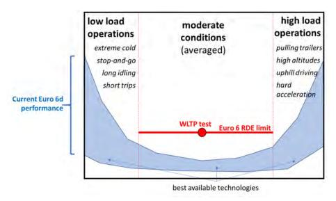
Figure 1.2: Graphic representation of current Euro 6d vehicle performance (blue band) in the context of RDE testing. The WLTP laboratory test is a very specific subset of moderate driving conditions (as indicated by the red dot). Comparatively, the RDE test addresses a much wider range of driving conditions (as shown by the red line), though these conditions could still, on average, be described as moderate.
