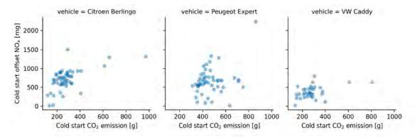
Figure 3.5: Cold start NO<sub>x</sub> emission of three Euro 6d diesel vehicles in relation to the cold start CO<sub>2</sub> emissions. Each dot represents the result of a single cold start.
