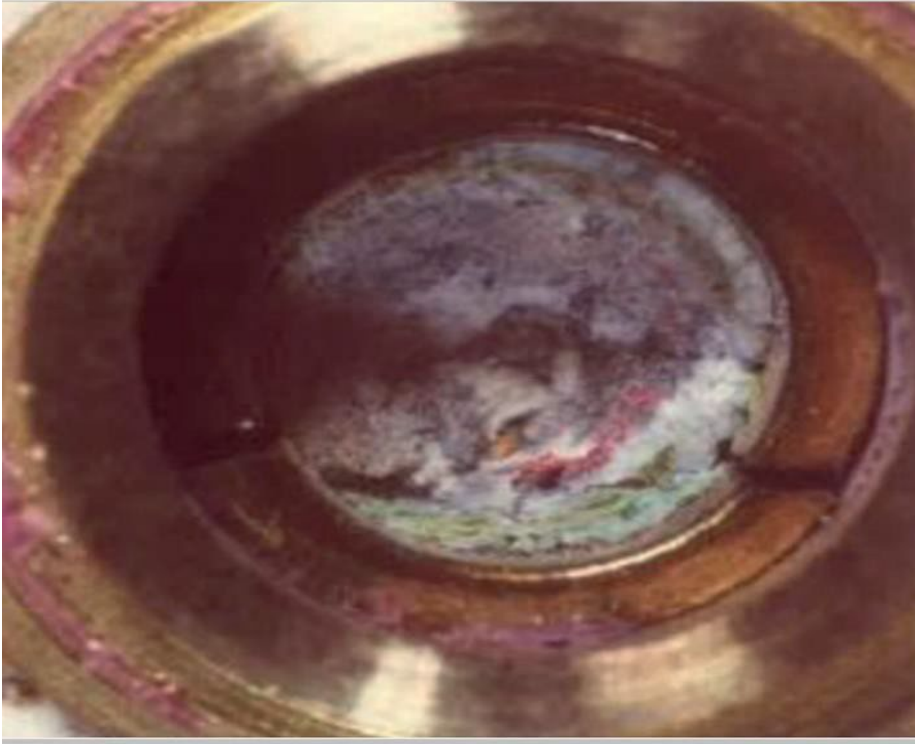
Figure 17: Top view of the aluminium detonator in the brass casing from fuze type V-19. Den Helder (1974) spontaneous reaction of corroded fuzes. (Picture: TNO)
