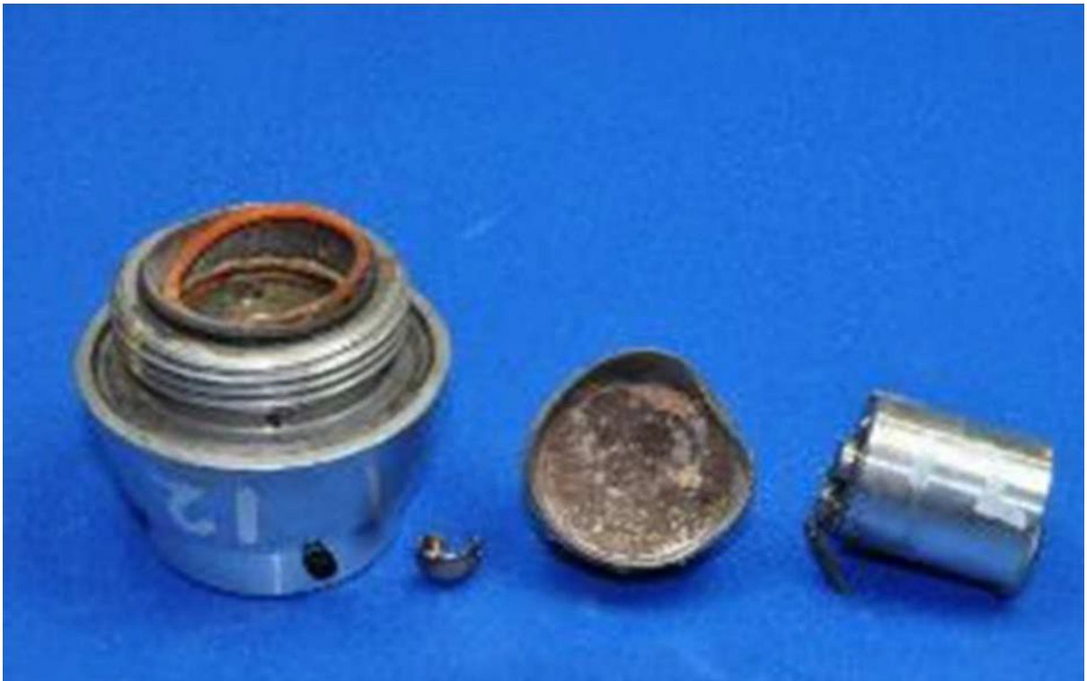
Figure 34: Explosive train interruption test carried out at 63°C by KC W&M. The booster charge has not detonated but it has fully combusted. In a higher confinement condition, as in an HE 80 round, transition to detonation may have occurred. (Picture: KC W&M)
