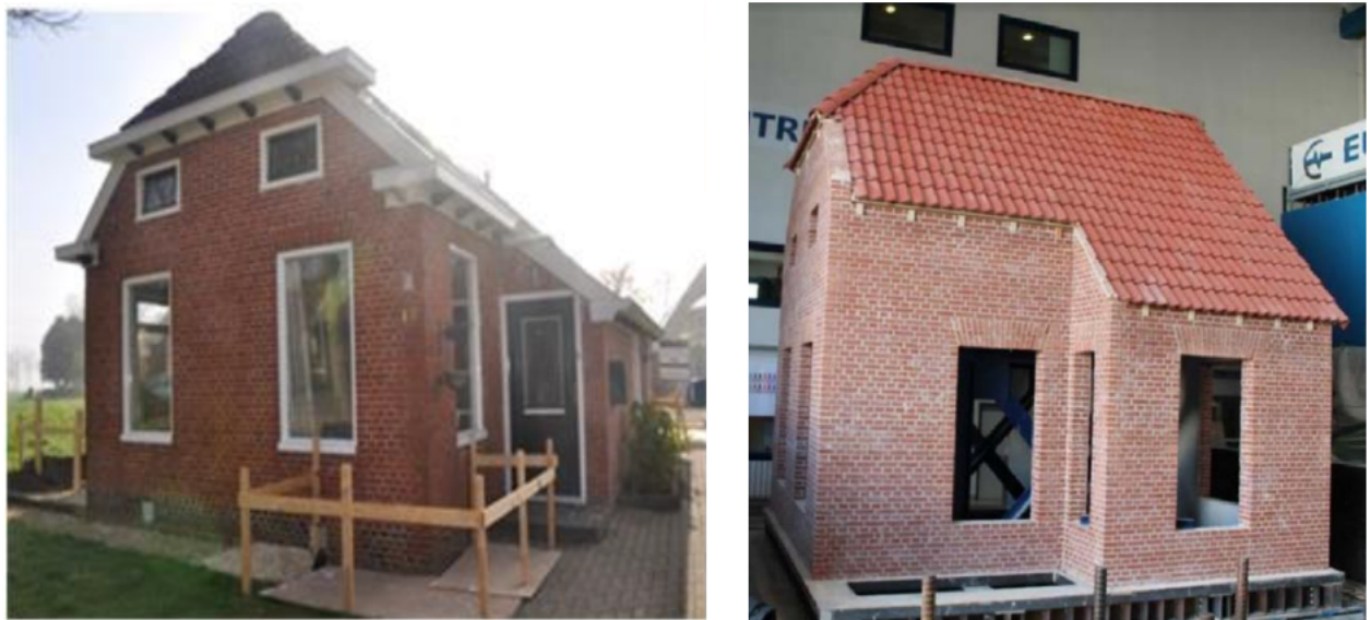
Figure 2: Buildings with construction details similar to those adopted for the shake-table test specimen (from [3]), and actual specimen tested at the laboratory of EUCENTRE (from [11]).
